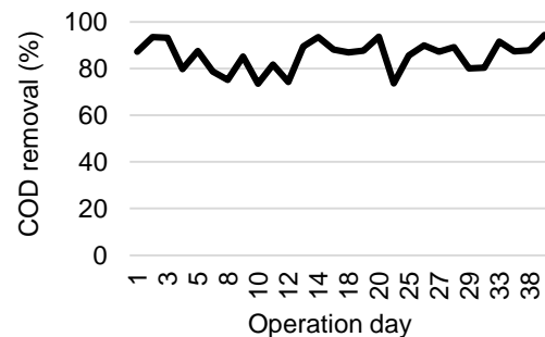
Fig. 2 Chemical Oxygen Demand removal by the activated sludge during the reactor operation using synthetic municipal wastewater
