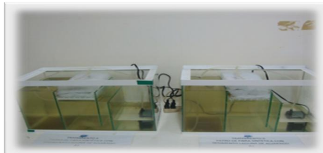
Fig. 1. Systems of microbial mats for the treatment of effluent from shrimp farming, small-scale laboratory.
